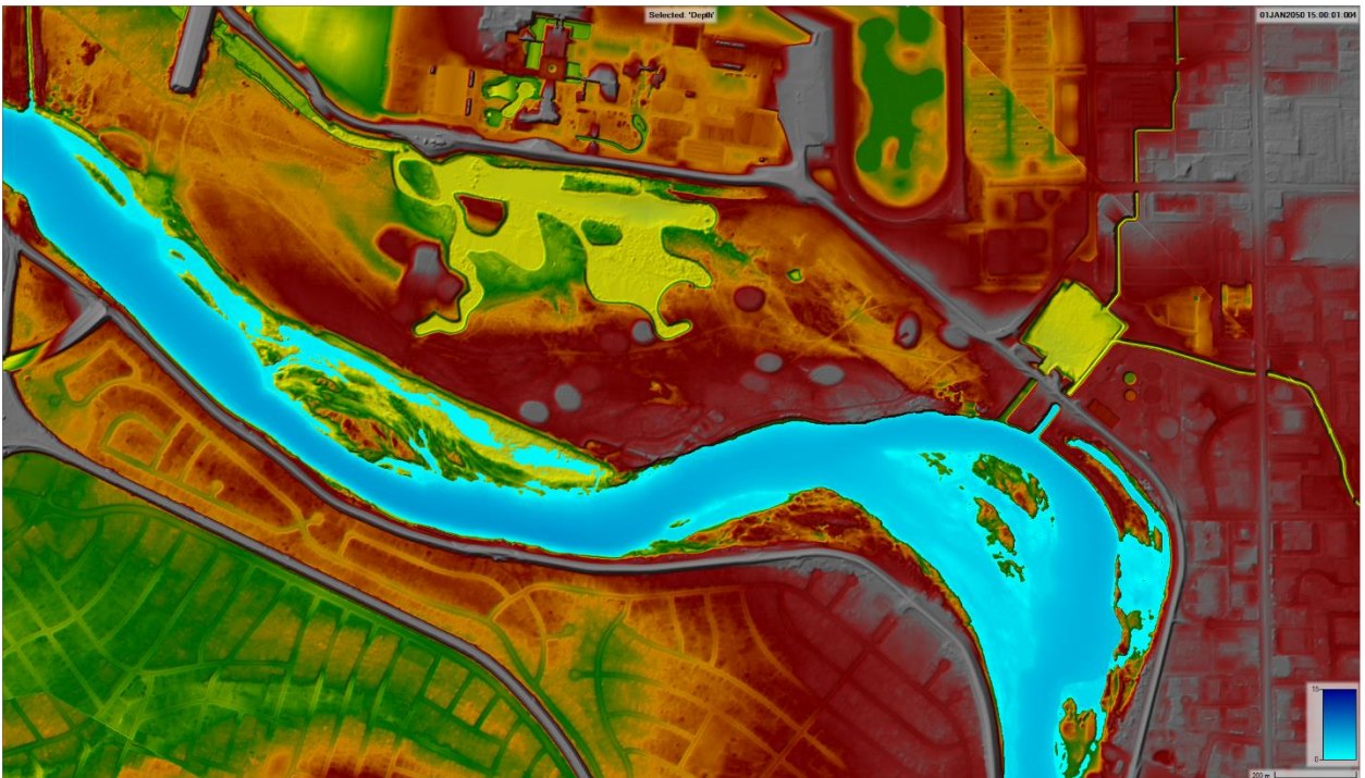
Figure 41. At 15 hours the channel has filled previously dry areas and is beginning to reach capacity.
