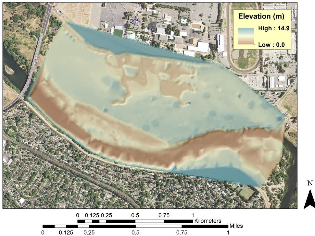
Figure 33. Digital elevation model of the floodplain remnant including Bushy Lake (light brown terrain in the middle of the map just south of Cal Expo)
